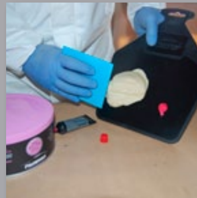
3 Mix the appropriate amount of ProWorx finishing filler at a ratio of 2% at an ambient temperature of 20°C.
